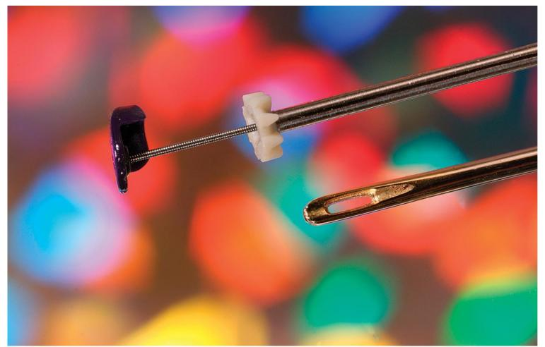
MICRO MATERIAL: The device is made from Ultem, an amorphous thermoplastic polyetherimide (PEI) resin. MICRO FEATURES: The overmolded assembly design has a spring OD of 0.11" (0.28mm). The Ultem wall thickness is 0.012" (0.30mm). DESCRIPTION: The assembly device and mating overmolded tube were components of an endoscopic suturing device used in a non-robotic, minimally invasive surgery. The laparoscopic procedure deployed a circular pattern of staples to create a closure.
