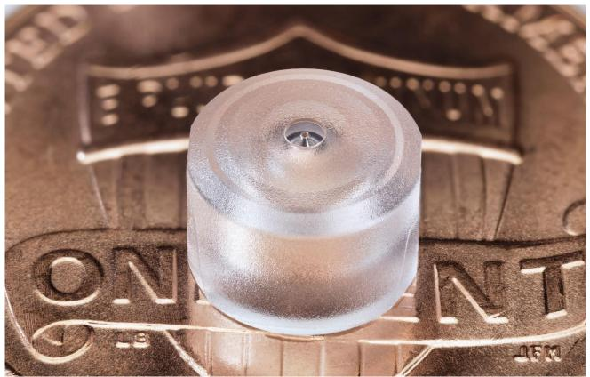
MICRO MATERIALS: This drug delivery device is made from Cyclo Olefin Polymer (COP).
