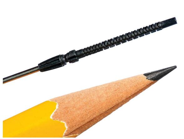
MICRO MATERIAL: This ablation tip is molded Glass Filled LCP (Liquid Crystal Polymer). MICRO FEATURES: The device design features 0.030" (0.76 mm) ID and 0.950" (24.13 mm) OAL. DESCRIPTION: The strain relief device has extremely long flow length; minimum wall thickness of 0.004" (0.10 mm).
