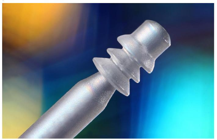
MICRO MATERIAL: Component made of polypropylene (PP) thermoplastic polymers. MICRO FEATURES: This plug is 0.079" (2 mm) diameter and 0.098" (2.5 mm) length DESCRIPTION: This tiny component plug is one of our many micro medical components that we painstakingly built from polypropylene. The micro insert
