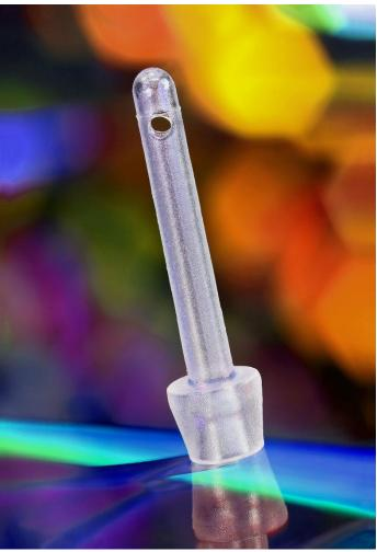
MICRO MATERIALS: The device is molded in PC (Polycarbonate), a thermoplastic material. MICRO FEATURES: The flow tube device OD is about .0065" and the ID is about .0046". The diameter of the hole is .033". DESCRIPTION: The flow tube device part is about 0.6" long.
