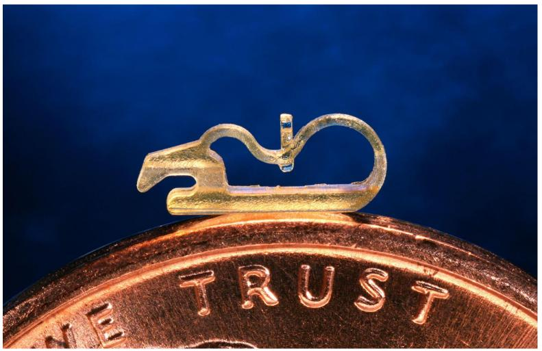
MICRO MATERIAL: The clip is made of Ultem 1010 thermoplastic resin. MICRO FEATURES: The clip component measures 0.009" (0.23 mm) in wall thickness.
