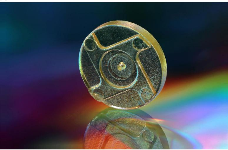
MICRO MATERIAL: The device is made of Ultem, an amorphous thermoplastic polyetherimide (PEI) resin. MICRO FEATURES: The design features a 0.0063" (0.16 mm) Nozzle ID. DESCRIPTION: The nozzle cover device's Nozzle ID is directly related to spray pattern.
