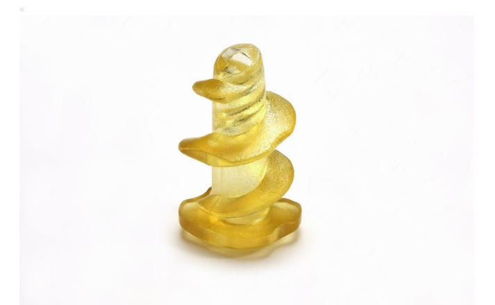
MICRO MATERIAL: The screw is made of Ultem, an amorphous thermoplastic polyetherimide (PEI) resin. MICRO FEATURES: The device features an end of flow, which is a feather-edge condition. DESCRIPTION: This design from our customer called for pushing a difficult flowing material to a feather-edge while maintaining exacting tolerances. The specifications for the screw required a very exact micro tooling design in a highly capable molding system.
