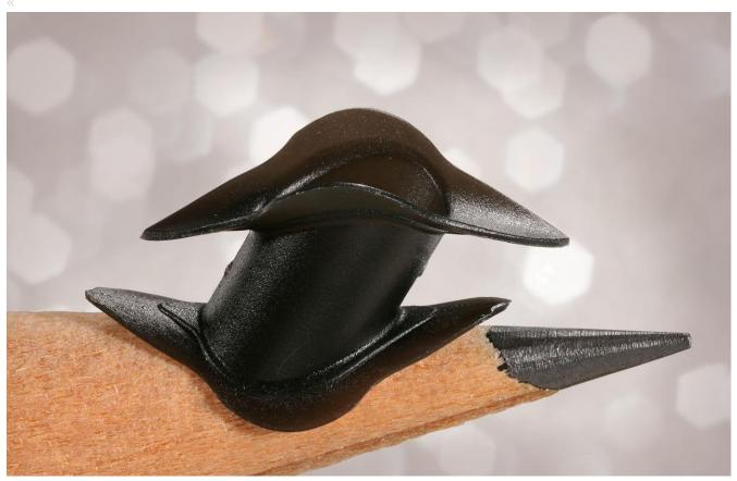
MICRO MATERIAL: The device is molded of confidential thermoplastic material. MICRO FEATURES: There isn't a straight line on this connector. Average wall thickness of 0.008" (0.20 mm). DESCRIPTION: The vascular connectors are surgical implants that form precisely controlled vascular connections while minimizing vessel trauma. Extremely challenging material, parts have very thin molded walls throughout (0.008").
