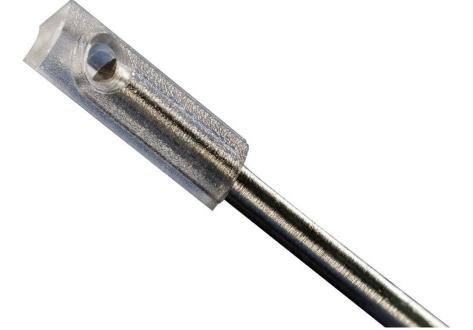
MICRO MATERIAL: The micro imaging tip device is made from PC, a thermoplastic polymer. MICRO FEATURES: The micro component stands 0.1" tall with a .002" wall thickness. DESCRIPTION: The micro imaging tip is about 1/4 the size of a grain of rice.
