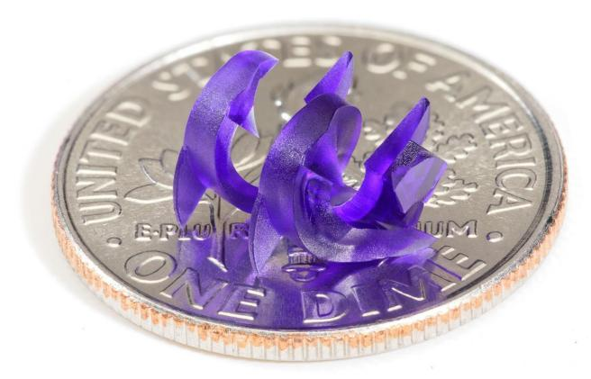
MICRO MATERIALS: This implantable tack is made of a bioabsorbable polymer.
