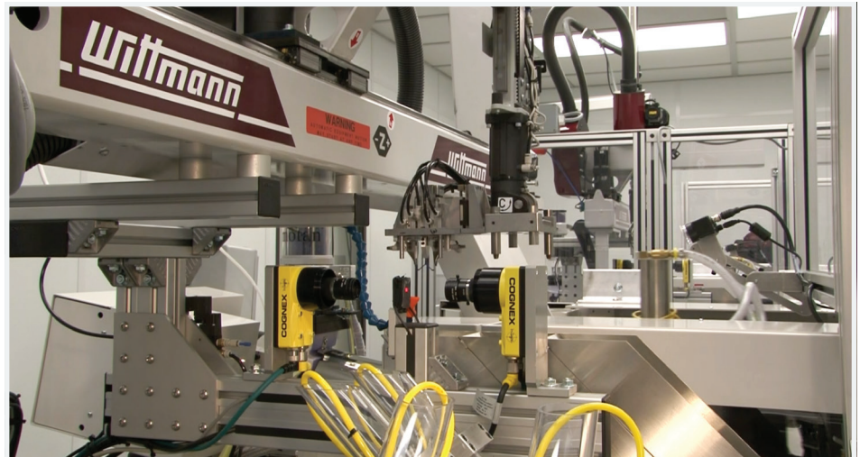
A standard molding cell at kunlun, equipped with custom end-of-arm tooling (EOAT), robotics, in-line camera systems, and automated part collection.
