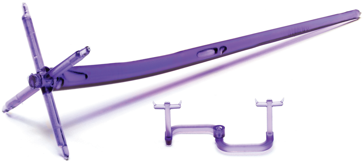
FIGURE 5: Typical runner (left) and optimized runner (right)
