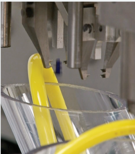
The custom EOAT drops a molded bioabsorbable component into the collection tube after passing camera inspection.
