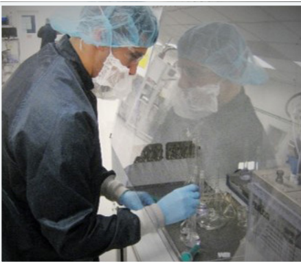
process engineer testing for Inherent Viscosity (IV).
